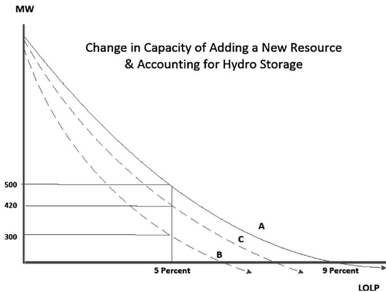
Fig. 4. Change in capacity from adding a new resource and accounting for hydro storage.
