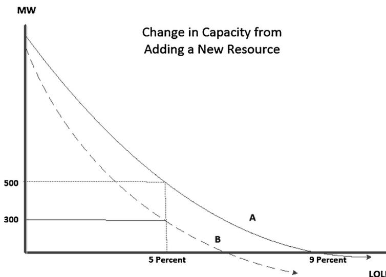
Fig. 2. Change in capacity from adding a new resource.
